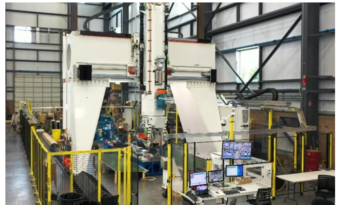
Figure 1. Electroimpact's 5-axis milling machine optimized for aerospace applications.
